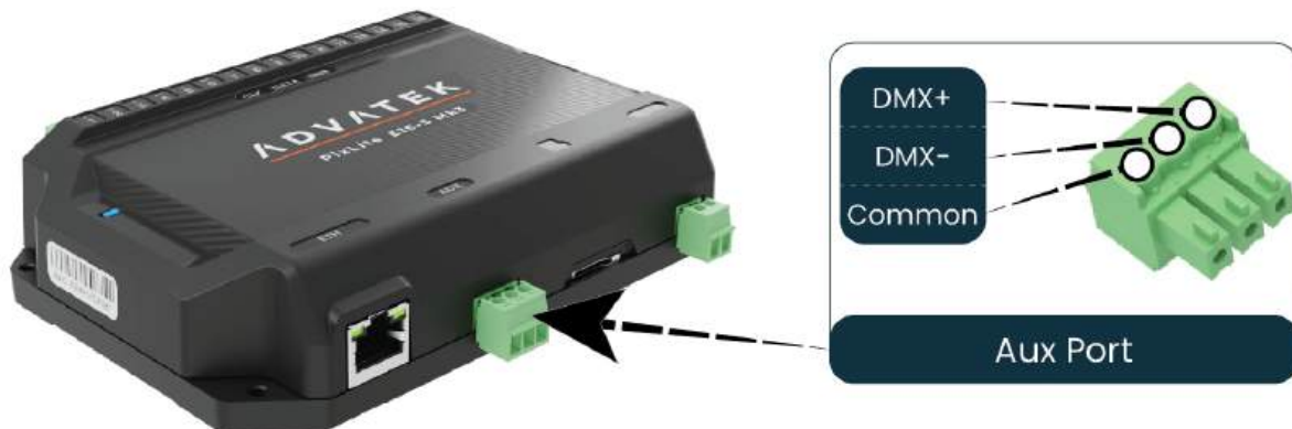
Figure 13: Location and Pinout of the Aux Port
