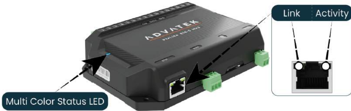
Figure 17: Location of LEDs
