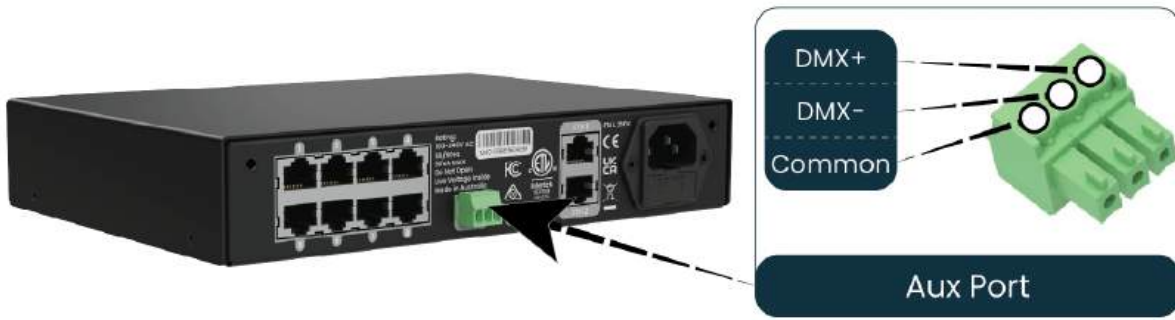
Figure 17: Location and Pinout of the Aux Port
