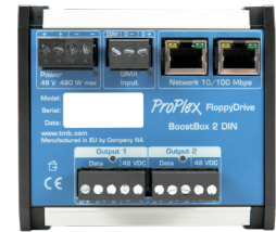
2-output DIN Rail Mount BoostBox with Pluggable Terminal Block BuckBoost Drive output connectors and dual Ethernet plus DMX control ports. (requires external 48V PSU)
