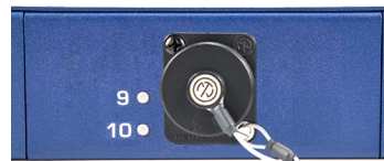
1x OpticalCON QUAD running ports 9-10
